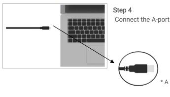
Connect the A-port of the USB 3.0 cable to the PC.
