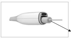
Step 2 Insert the battery at the bottom of the handpiece.
