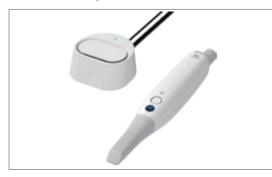
Once it is turned on, the i700 wireless will try to automatically pair with the hub. For a fast pairing, both the i700 wireless and the hub must be powered and placed near each other.
