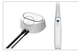
When pairing is in progress, the LED on top of the i700 wireless blinks. Once the pairing is complete, the LED lights up. You can now start scanning.
