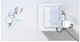
There should be no obstruction between the i700 wireless and the wireless hub. It is also recommended to have the hub and the transmitter of the handpiece face each other's direction when working.
