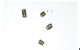
Figure 8. Three fractured prosthetic screws retrieved successfully (one of the screws had broken into two pieces).
